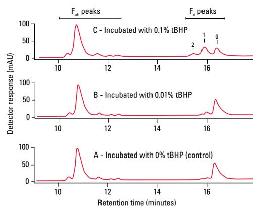
Column: **TSKgel Butyl-NPR, 2.5 µm, 4.6 mm ID × 3.5 cm**
