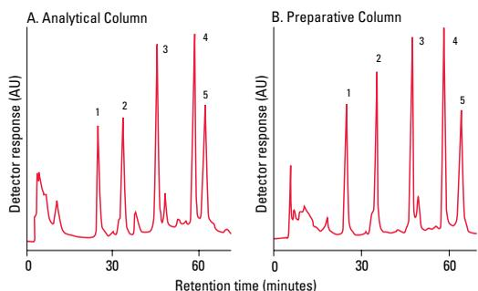
Columns: **A: TSKgel Phenyl-5PW, 10  $\mu$ m, 7.5 mm ID  $\times$  7.5 cm**
