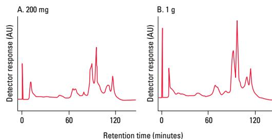
Columns: **A: TSKgel Phenyl-5PW, 13  $\mu$ m, 21.5 mm ID  $\times$  15 cm**
