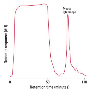
Column: **TSKgel Ether-5PW, 10 μm, 8.0 mm ID × 7.5 cm, glass**
